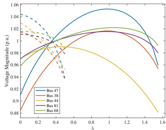
Fig. 6. CPF results for the weakest buses before (dashed lines) and after (solid lines) applying the proposed method to the first scenario for the IEEE 118-bus case.
