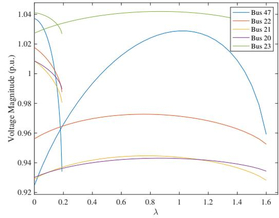
Fig. 8. CPF results for the weakest busses before (dashed lines) and after (solid lines) applying the proposed method to the second scenario for the IEEE 118-bus case.
