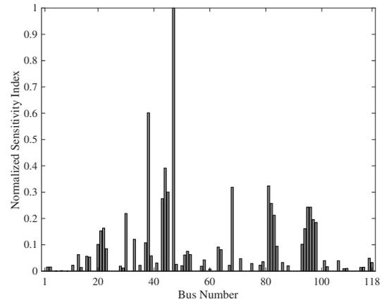
Fig. 5. Bus sensitivities after a contingency on the line between buses 69 and 75 in the first scenario for the IEEE 118-bus case.
