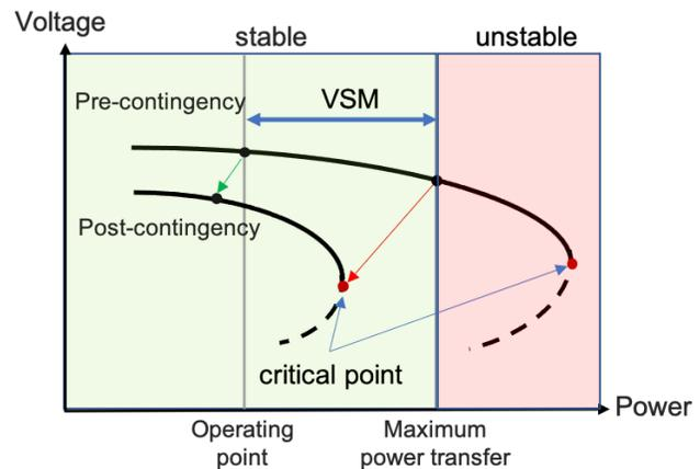
Fig. 1. Active power voltage curve showing the critical point pre- and post-contingency.
