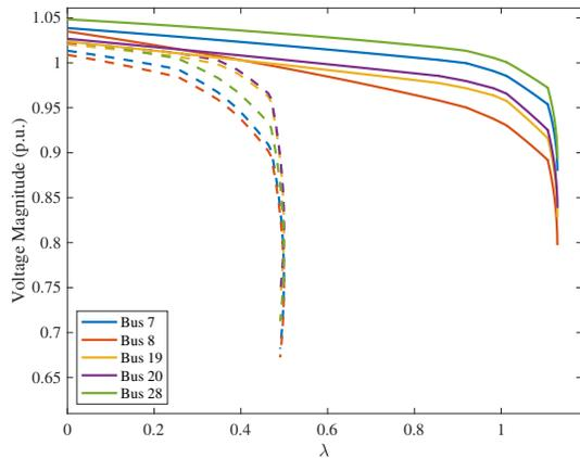
Fig. 4. CPF results before (dashed lines) and after (solid lines) applying the proposed method for the IEEE 30-bus case.
