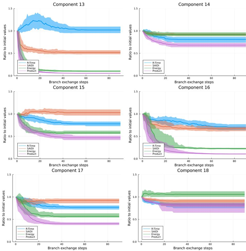
FIG. 9. R-TIME, SAIDI, energy, and product objectives for Greensboro components 13-18 during the branch exchange local search. Objectives are plotted as a ratio of their value after each step to the initial values, and each plot shows the median values and percentiles (first to last deciles) for each objective, taken over 50 applications of the branch exchange local search on the component.
