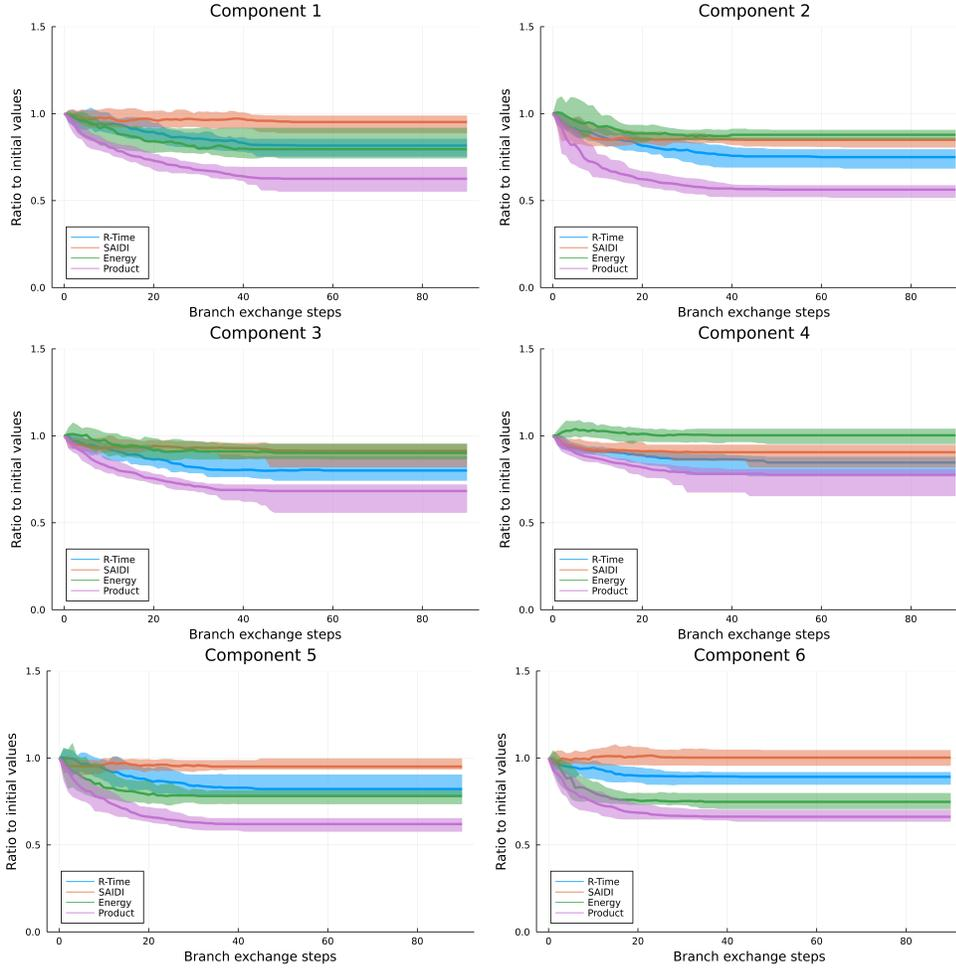
FIG. 7. R-TIME, SAIDI, energy, and product objectives for Greensboro components 1-6 during the branch exchange local search. Objectives are plotted as a ratio of their value after each step to the initial values, and each plot shows the median values and percentiles (first to last deciles) for each objective, taken over 50 applications of the branch exchange local search on the component.
