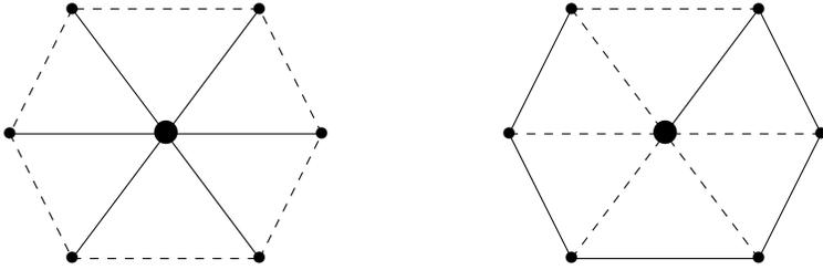
FIG. 1. Two spanning trees on the same network. Solid edges are in  $T$ , dashed edges are in  $E \setminus T$ , the source  $r$  is the largest vertex, and all vertex weights and edge failure probabilities are equal.
