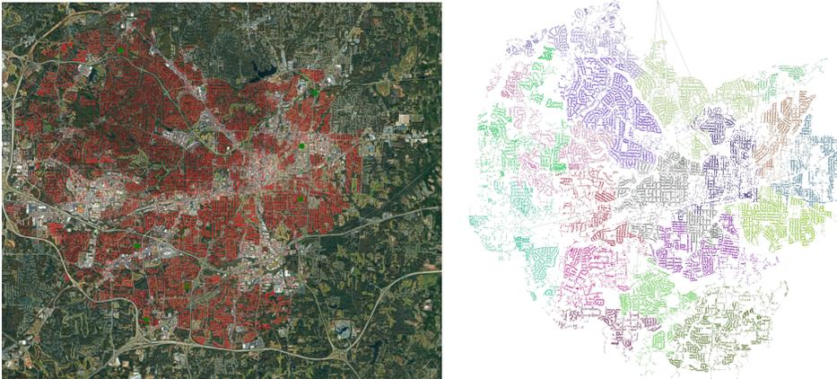
FIG. 4. (left) Buses shown on a satellite image of Greensboro, NC. (right) Each color is a different connected component in the graph where all the switches (black edges) are removed.
