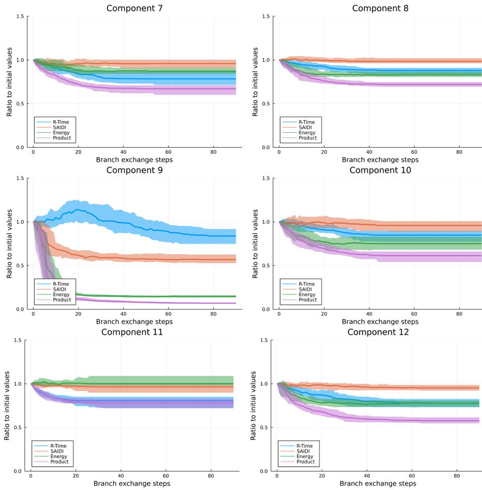
FIG. 8. R-TIME, SAIDI, energy, and product objectives for Greensboro components 7-12 during the branch exchange local search. Objectives are plotted as a ratio of their value after each step to the initial values, and each plot shows the median values and percentiles (first to last deciles) for each objective, taken over 50 applications of the branch exchange local search on the component.
