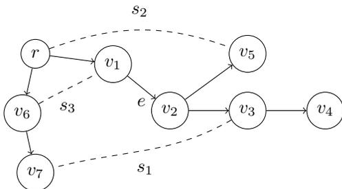
FIG. 2. An example of a network comprising a spanning tree (solid edges) and switches (dashed edges.)
