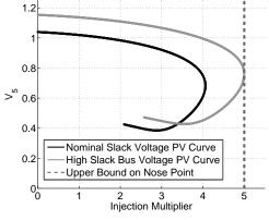
(b) Nominal and High Slack Bus Voltage PV Curves
