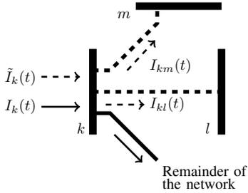
Fig. 2. Illustrative example of adjusting historical operational data to account for out-of-service lines. Lines  $(k, m) \in \mathcal{L}^-(t)$  and  $(l, k) \in \mathcal{L}^-(t)$  are out-of-service at time  $t$ . The solid arrows represent the currents associated with the in-service lines. The dashed arrows represent the currents which would have been induced by the historical voltage phasors if the out-of-service lines had been in-service at time  $t$ . (See equations (3) and (4).)
