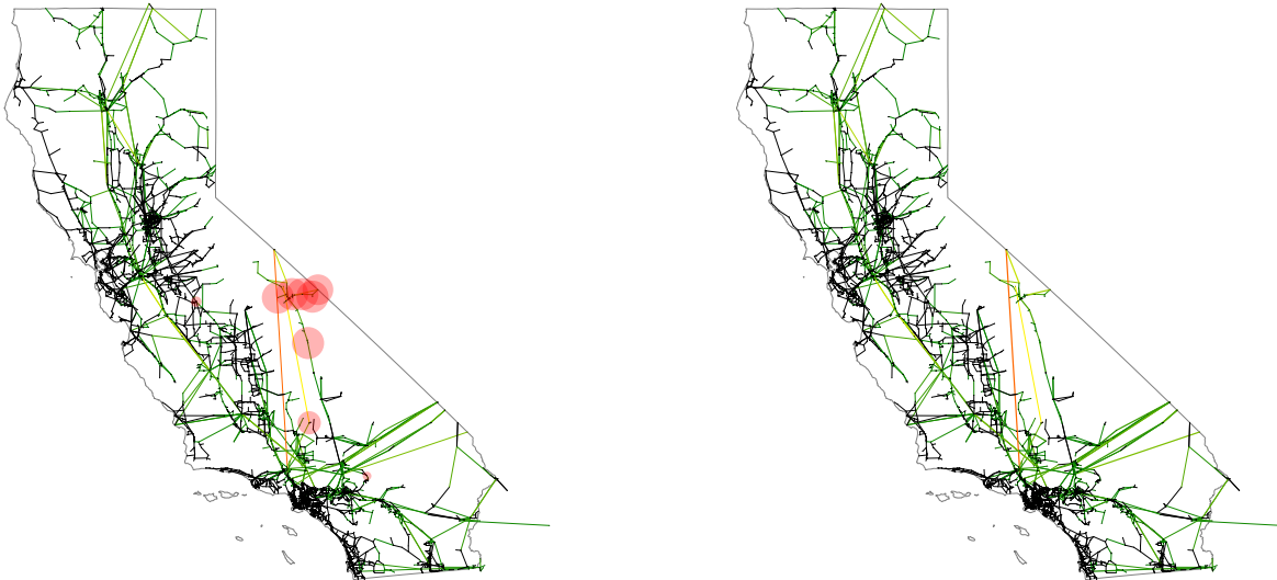
(a) Battery-only placement results (scheme 1) for the spring season. The size of the circle corresponds to the capacity of the installed battery with the largest circle equating to 400 MWh of installed capacity.
